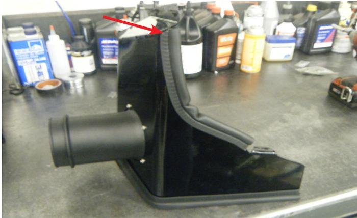
12. Firmly push the supplied shorter edge seal with the angle cut on one end onto the bottom of the airbox. The angle cut in the edge seal should be pointed down when the airbox gets installed into the vehicle, as shown by the arrow.
