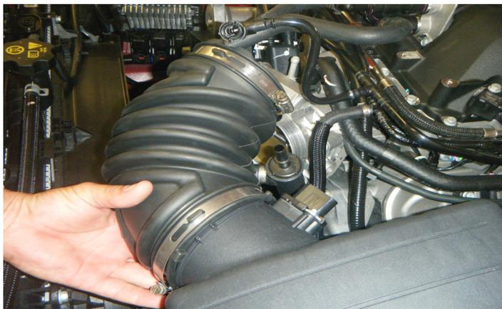
8. Using a 7mm socket, remove the two (2) screws that secure the MAF sensor to the airbox. Make sure to keep the stock MAF sensor as it will be re-used for the new air intake installation.
