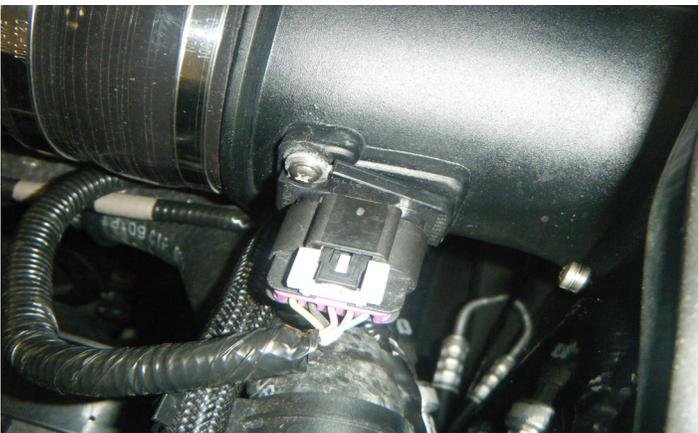
20. Connect the MAF sensor harness connector to the MAF sensor housing. You should hear a click when the connector is fully engaged. Slide the grey tab to lock the MAF sensor connector in place.
