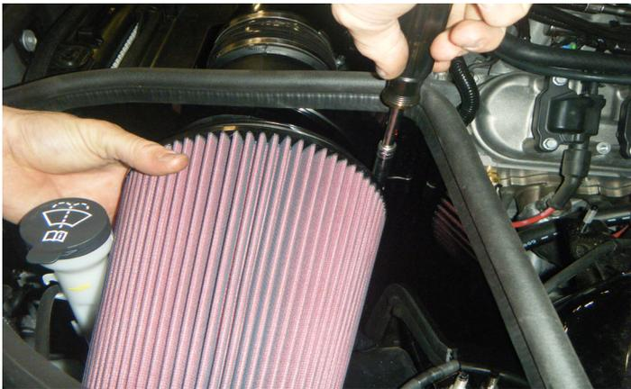
23. Carefully install the supplied air filter onto the MAF housing inside the airbox. If the airbox flange nut was left loosened, you can move the airbox slightly towards the passenger side of the vehicle to make installation of the air filter easier. Secure the air filter to the MAF housing using the large supplied worm clamp and an 8mm socket. Do not overtighten.
