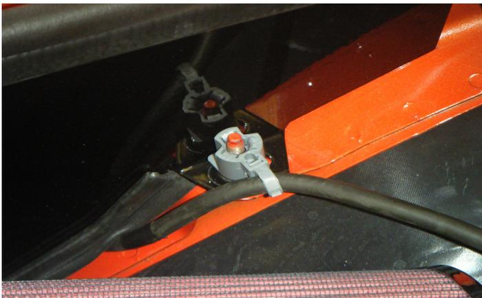
24. Tighten the airbox flange nut and then attach the ground wire guide back onto the upper stud as well.
