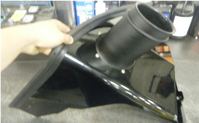
11. Firmly push the supplied longer edge seal onto the top of the airbox.
