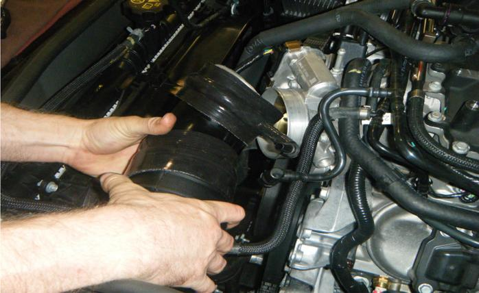
17. Insert the supplied 45 degree breather hose adapter into the supplied hump hose with built-in breather. Clock the adapter so that it points straight up, as shown in the picture.
