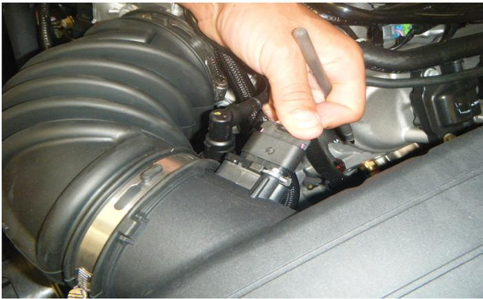
3. Unplug the Mass Air Flow (MAF) connector, which is located on the side of the airbox inlet, by first sliding the grey tab to unlock the connector. Then, press on the center tab and pull the connector away from the airbox inlet.
