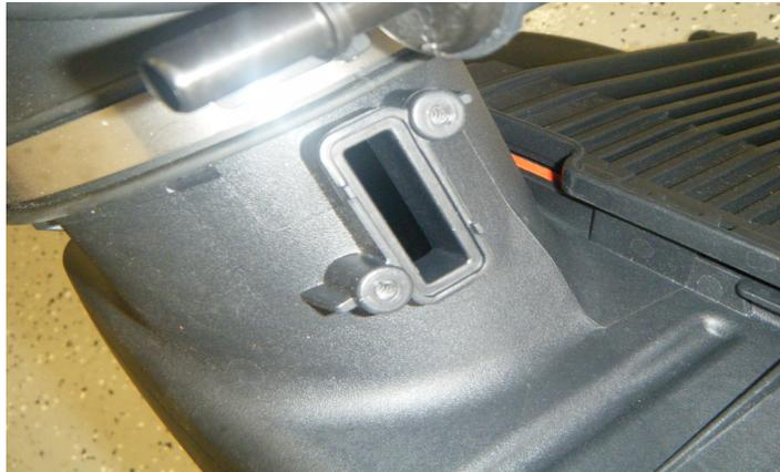
9. Using a phillips head screwdriver, insert the supplied MAF housing through the hole in the supplied airbox. Using the five (5) 10-32 screws, secure the MAF housing to the airbox. The screws should be tightened in a star pattern with the screw behind the MAF sensor being the first to be tightened.
