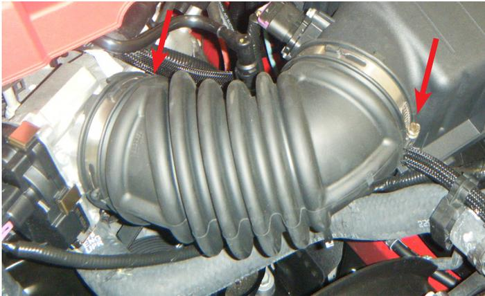
4. Loosen the hose clamps holding the air intake tube to the throttle body and airbox using an 8mm socket.
