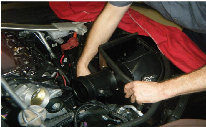
13. Lower the airbox assembly into lowering the airbox onto the bottom grommet and the upper stud as shown the illustration. Firmly push down on the airbox to verify that the airbox is fully seated onto the grommet.
