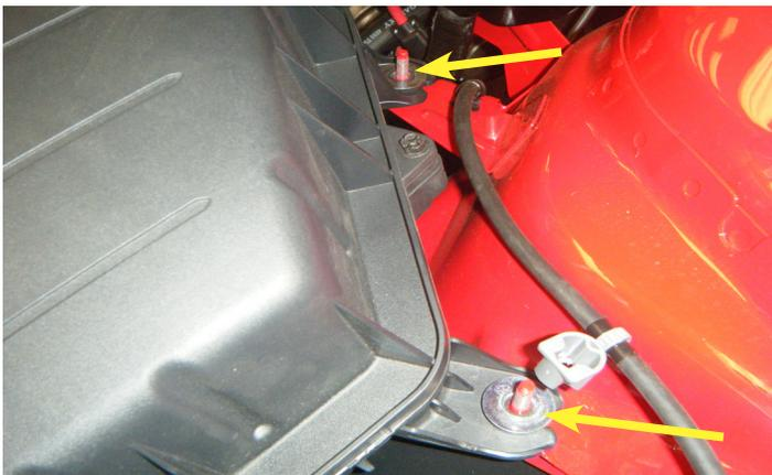
5. Remove the two (2) nuts that hold the airbox in place using a 10mm deep socket.
