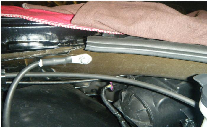
22. Using a 10mm socket, install the supplied ground bolt allowing additional clearance for the air filter. Torque the bolt to 89 in-lbs.
